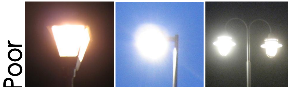
Unshielded Pole Mounted Fixtures (High Potential for Glare / Light Pollution)
